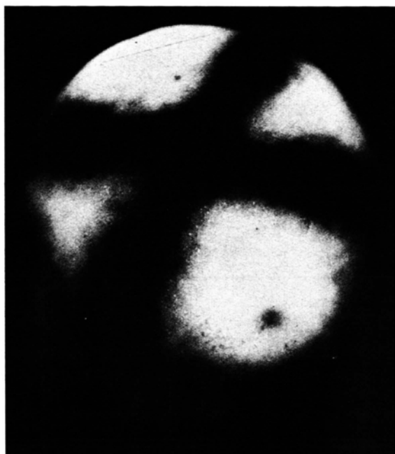
Fig. 5. FEM picture of a W tip.
